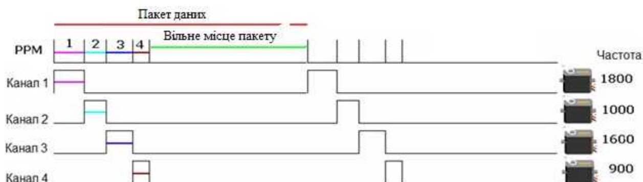
Figure 38. Graphical representation of the PWM signal transmitting signals from four control channels in a single packet.
