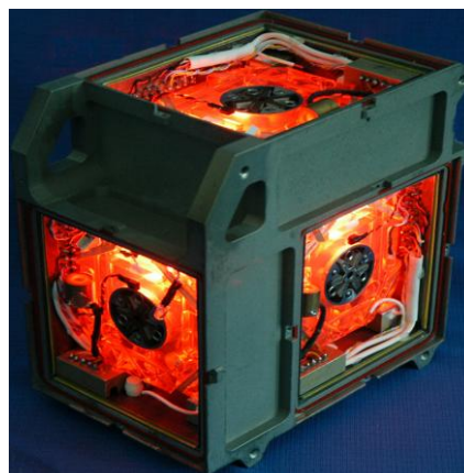
Fig. 1.3.6. Inertial Measurement Unit Based on Four-mirror RLG With Dithers
