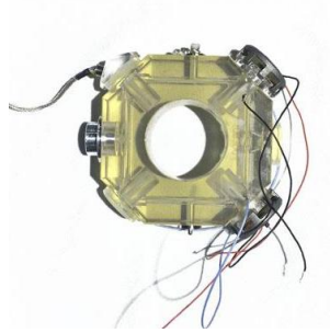
Fig. 1.3.7. JG132 Three-axis monolithic ring laser gyroscope
