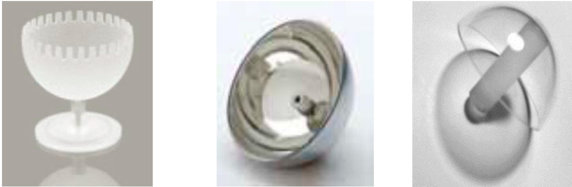
Fig. 1.5.2. Resonators made of fused quartz: a) a glass with 32 teeth; b) a mushroom-shaped resonator coated with a chromium film; c) a resonator assembled with a stem by deep optical contact
