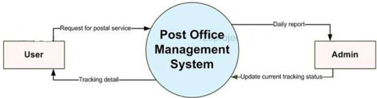
Figure 3.4 – Level 0 DFD for Post Office Management System [3]
